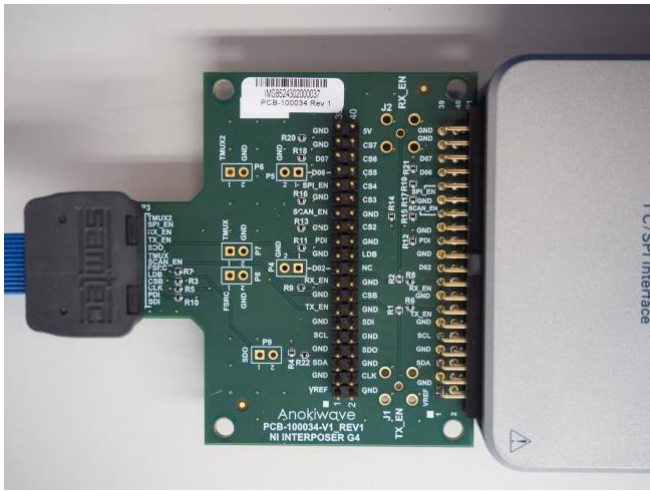
Figure 20: Connect IO Cable to P3 on Interposer Board (P6 TMUX2 pin can be used to monitor the PLL lock detect signal)
