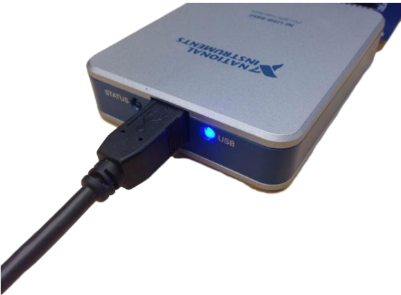
Figure 14: Connecting the NI-8452 to the PC Should Result in the USB Indicator Being Lit
