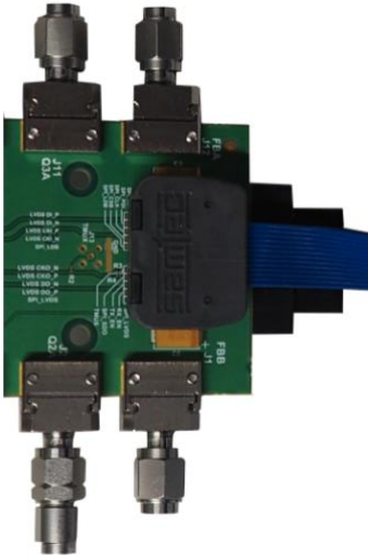
Figure 19: Connect IO Cable to P1 on Evaluation Board
