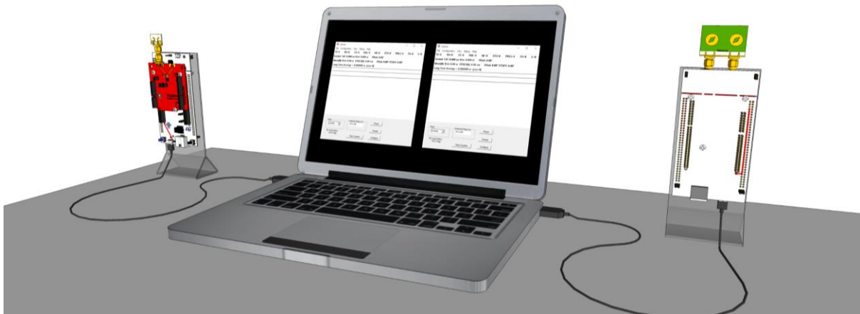
Figure 14 - Start the second DecaRanging-PC for TAG board and it also will start in listener mode.
