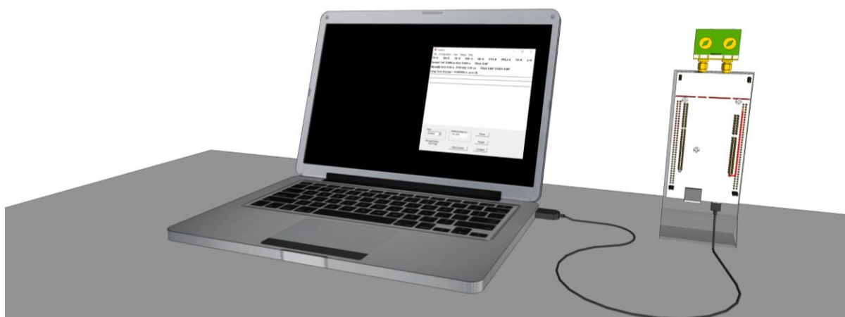
Figure 11 - Connect the NODE to the PC and start DecaRanging-PC
